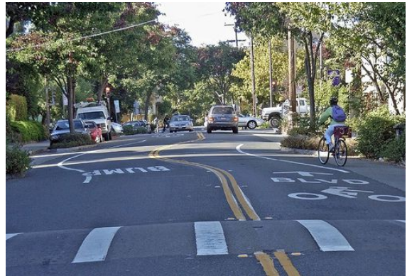
Bike route with chicanes to slow traffic flow. Source: Urban Street Design Guide, National Association of City Transportation Officials.
