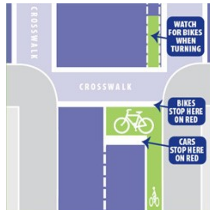
Bike lane with a bike box to let bicyclists queue in front of turning vehicles.
