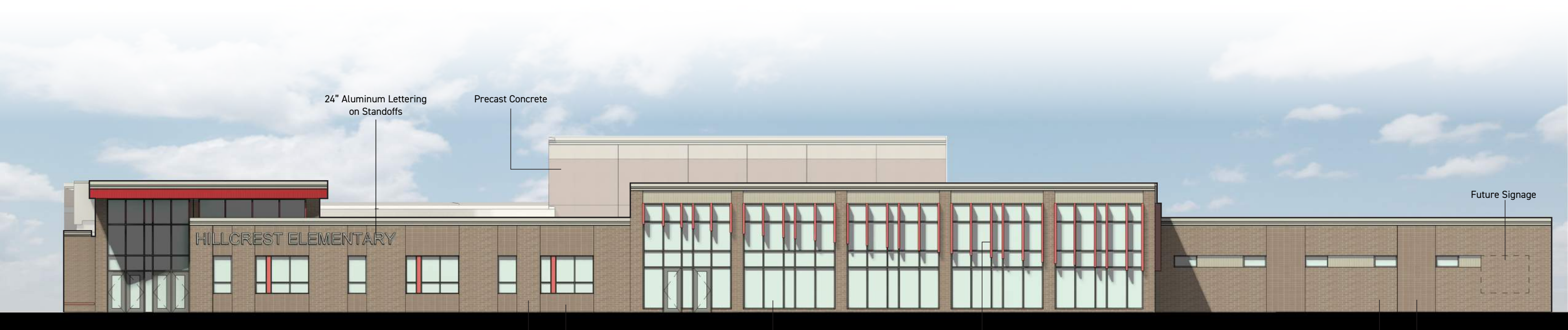
2 RE 1.0 ENTRY & CAFETERIA ADDITION Scale: 1/16" = 1'-0"
